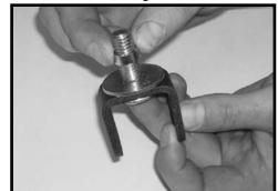
stock sway bar and secure using the new hardware. Make sure to use loctite and torgue to 70 ft lbs. Special note:
