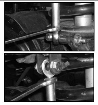
11. Locate (1) S10194 conned sleeves and (1) 1/2" unitorque 13. Repeat steps 3 - 12 on the passenger side of the vehinut from hardware bag 30927NB1. Install the new end link cle.
