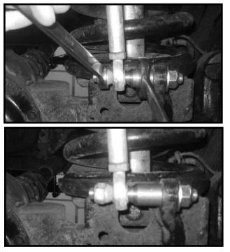
12. Move back to the nuts on the hiem joint and tighten up tight with the new center portion of the end link.
