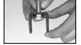
4. Locate (1) 9/16" flat washers from hardware bag 30927NB1 and install it on the new carriage bolt.
